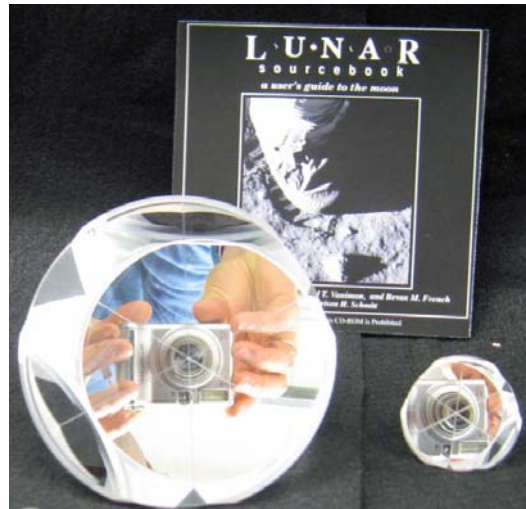
Figure 12: Photos of Apollo, 1 st generation and MoonLIGHT/LLRRA21, 2 nd generation CCR.
